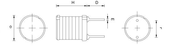
Dimensions do not include the solder on the terminal pins.
